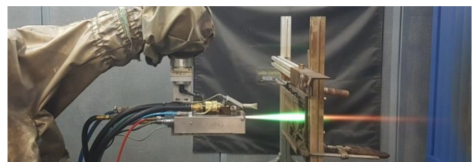
Thermal spraying of tin bronze
